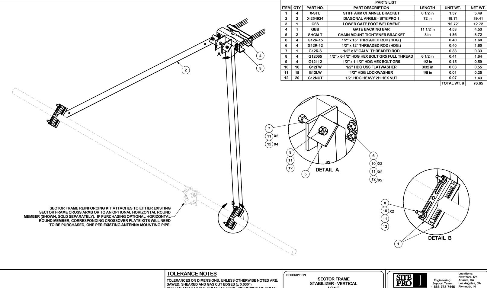
DRILLED AND GAS CUT HOLES (± 0.030") - NO CONING OF HOLES LASER CUT EDGES AND HOLES (± 0.010") - NO CONING OF HOLES BENDS ARE ± 1/2 DEGREE
